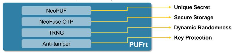
By integrating the PUFrt into the security subsystem, it can effectively manage the long and complex keys required for PQC algorithms.
