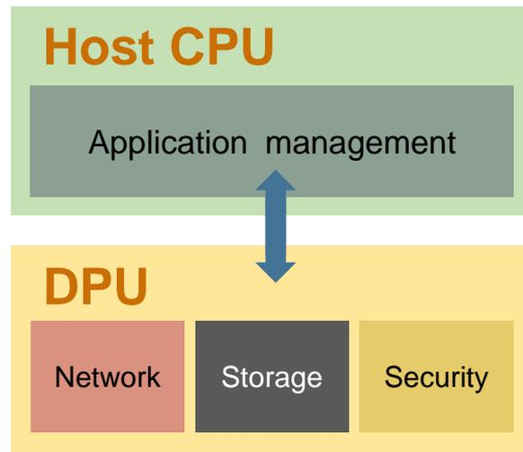
Offloading tasks to the DPU eases the workload of CPU and improves overall performance.
