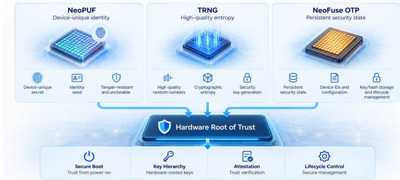
Figure 3. NeoPUF, NeoFuse OTP, and TRNG are complementary foundations for a hardware Root of Trust.
